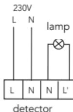
With this connection, the light fixture is controlled by the detector. All motion within the area covered by the detector triggers the light.
