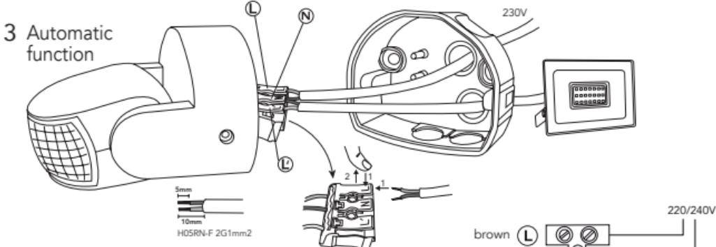
With this connection, the light fixture is controlled by the detector. All motion within the area covered by the detector triggers the light.
